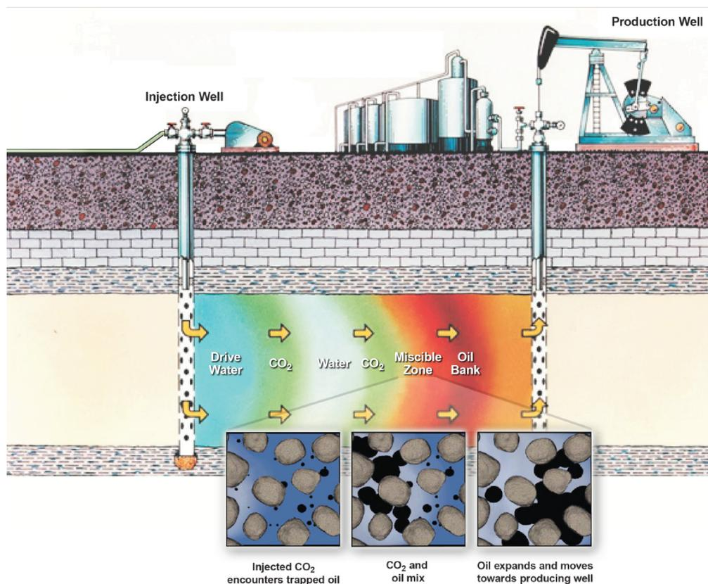
Figure 2. Enhanced Oil Recovery using CO<sub>2</sub> (water alternating gas) (5).
